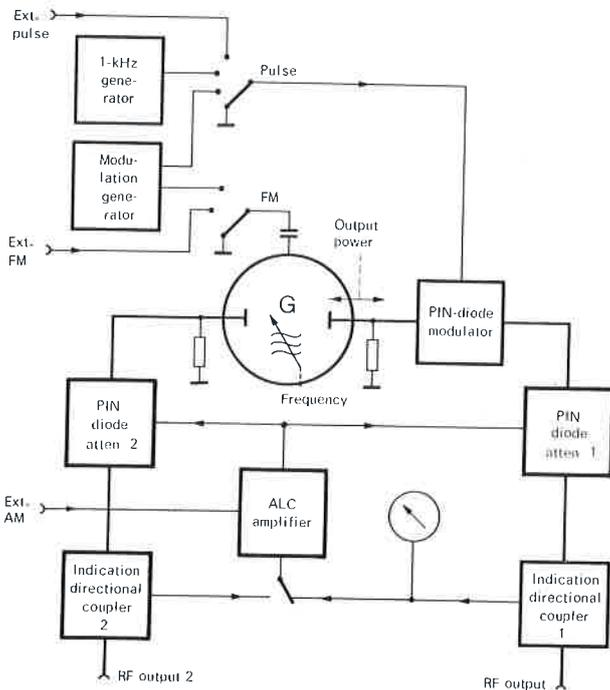
Block diagram of the SMAI with modulation unit
