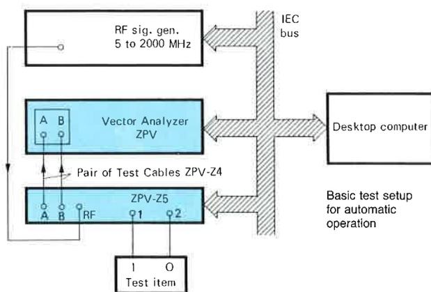
**Connections, settings, measurements.** The Test Adapter is connected to the RF generator and to channels A and B of the Vector Analyzer (see above). The test item input and output are taken to ports 1 and 2 of the ZPV-Z5.
