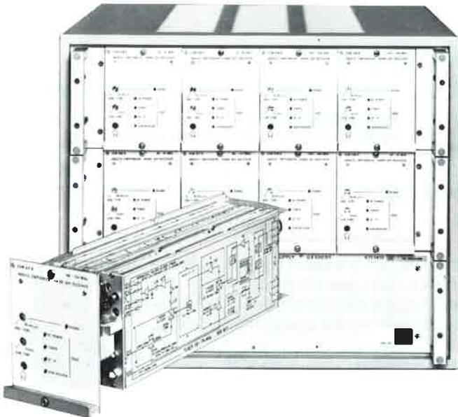
Eight hand-off receivers including power supply in a 19" cabinet
