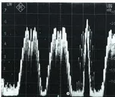
IF analysis: Modulation spectrum of one occupied and three free public-land-mobile-service channels; display width 200 kHz, resolution 1.5 kHz
