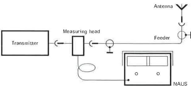
Power measurement on antenna feeder using NAUS
