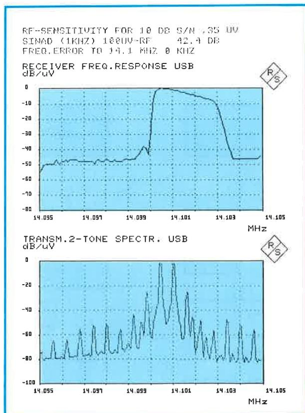
Test results: sensitivity measurement (top) and SSB two-tone measurement using Sideband Mixer Plug-in ATS-SM (bottom)
