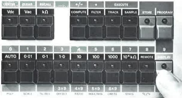
Panel controls for manual measurements, e.g. display and scale length (3×9 to 6×9) as well as integration time
