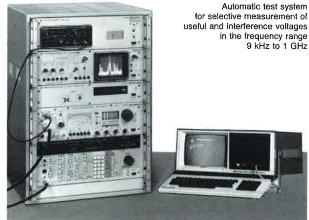
Automatic test system for selective measurement of useful and interference voltages in the frequency range 9 kHz to 1 GHz
