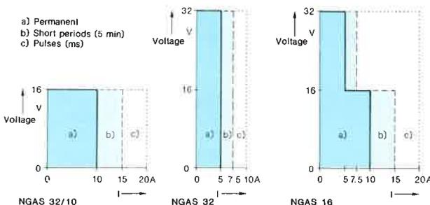
Current drain of NGAS as a function of output voltage
