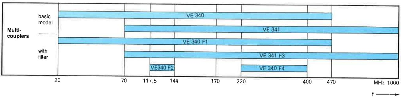
The broadband **Multicouplers VE 340** (20 to 470 MHz) and **VE 341** (70 to 1000 MHz) permit **up to eight receivers** or – via an inserted DC feed unit – further multicouplers with as many subsequent receivers to be simultaneously operated from one antenna. For operation without preceding Preamplifiers VE 031 to VE 034, these multicouplers are available with filters for limiting the frequency range (see specifications).
