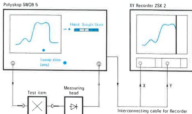
Logging of test results in single sweep (sweep time about 30 s) using XY Recorder ZSK 2
