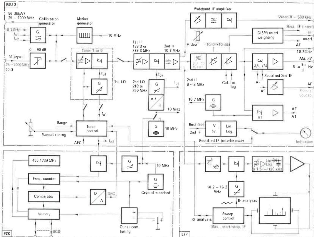
Block diagram of VHF-UHF Selective Test Equipment MSU
