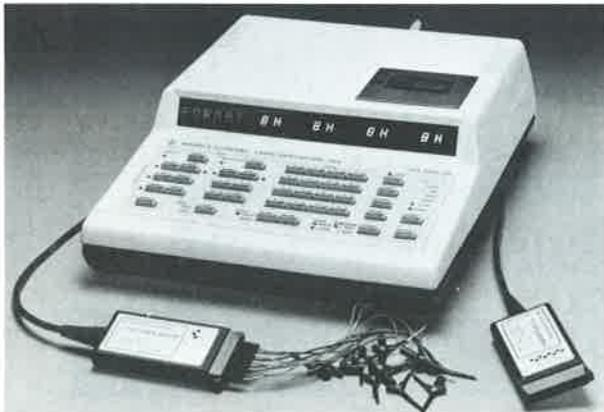
Logic Generator IGA with clock driver (including driver adapter, cable and mini-clips) and data driver
