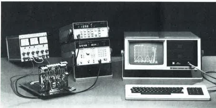
Automatic filter measurement with RMS Voltmeter URE, Process Controller PUC and Generator SPN
