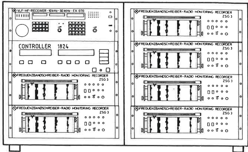
The **Automatic RF Spectrum Occupancy Recording Equipment EA 110** and **EA 115** measure and record the occupancy of frequency bands over extended periods of time. The recordings clearly show any unduly high or low signal density at certain frequencies and times. With suitably adjusted sweep width and resolution, the plotted graph can also provide information on the frequency stability, type of modulation and class of emission of the transmitters observed.
