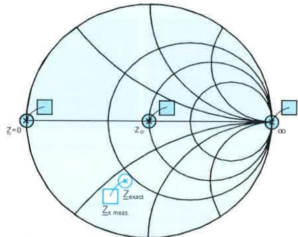
Three-point error correction at frequency  $f_1$
