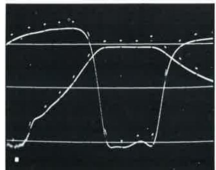
Reflection-coefficient and attenuation curves of 25-MHz bandpass filter with pulse frequency markers
