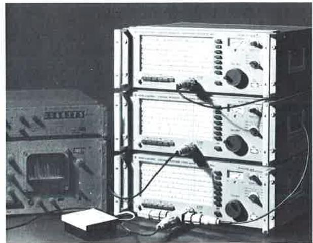
Power Signal Generator SMLU (see page 70) used in test setup for crossmodulation measurement
