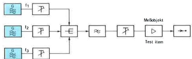
Principle of test assembly for intermodulation and crossmodulation measurements using the three-signal method
