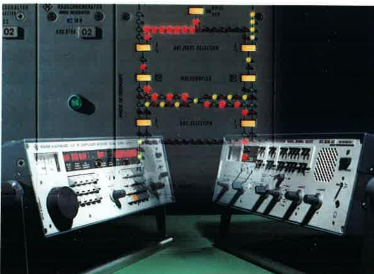
Remotely controllable VLF-HF receiving system made up of the Receivers EK070 and EK071
