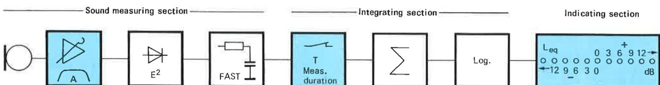
These limits are the centre values of the ELDO 4 subranges. A symmetrically arranged LED scale (red for + and green for -) directly indicates the amount by which the measured value is above or below the selected noise limit. The measured value is always to the right of the indicated figure. If, for example, +6 dB is indicated and the range selected is 70 dB, the measured value is above 76 dB, more precisely between 76 and 79 dB.
