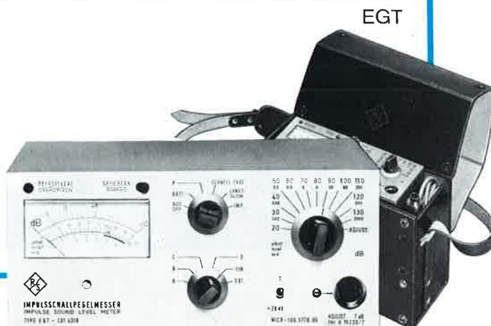
The portable **Impulse Sound-level Meter EGT** covers the wide test range of 24 to 160 dB and fulfils the requirements of the German Standard DIN 45 633, sheet 1, for precision sound-level meters, and sheet 2 for impulse sound-level meters, and of IEC 651 Type 1.
