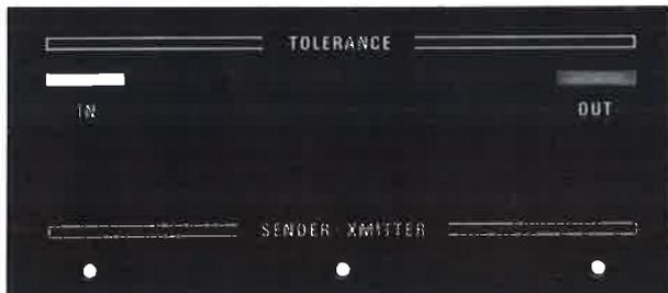
Light bars for performance assessment of the transceiver upon completion of the automatic test
