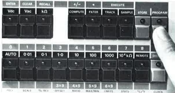
Keyboard offers wide range of input, output, calculation and storage functions
