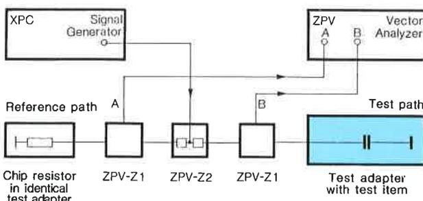
Block diagram of RF-component tester for capacitors
