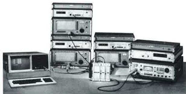
Automatic test assembly for intermodulation and crossmodulation measurements (see page 116)
