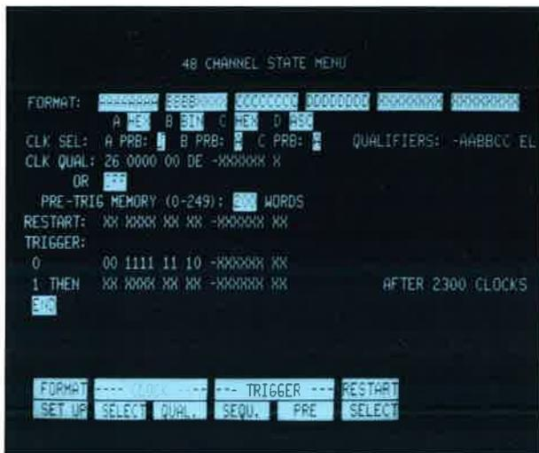
Basic menu of 48-channel logic analyzer
