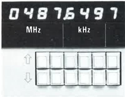
Keys associated with the various digits permit stepwise or continuous variation of numerical values entered (e.g. frequency as here displayed)
