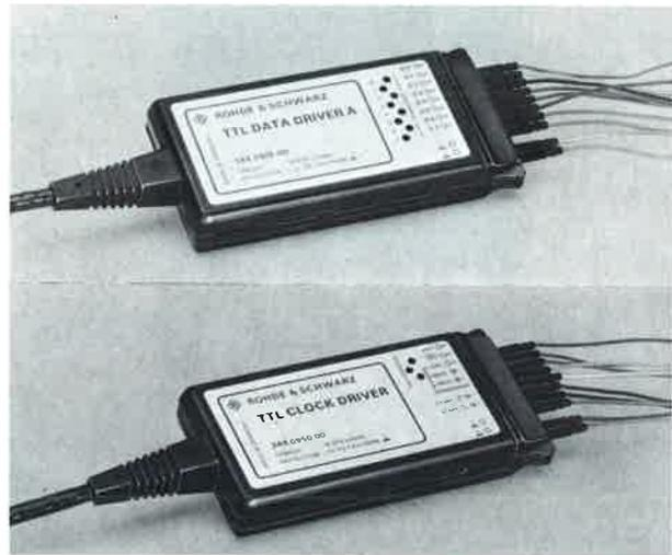
TTL Data Driver IGA-Z4 (top) and TTL Clock Driver IGA-Z5 (bottom)
