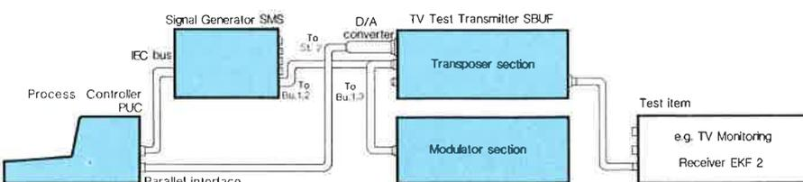
Block diagram of computer-controlled test assembly for rapid channel change, the reference frequency is delivered by the Signal Generator SMS and the tuning voltage produced by a D/A converter (e.g. Motorola MC 1408)
