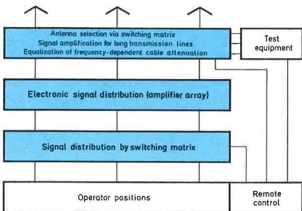
Principle of a system for distribution and transmission of antenna signals in short-, medium- and longwave receiving systems
