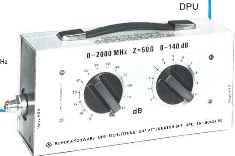
The **UHF Attenuator Set DPU** is simple and convenient in use over its frequency range from DC to about 2 GHz. Its applications include primarily attenuation measurements and gain measurements as well as accurate adjustment of very low voltages.
