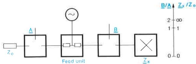
Result from  $B/A$  ratio measurement as a function of impedance  $Z_x$  (in reflection measurement)
