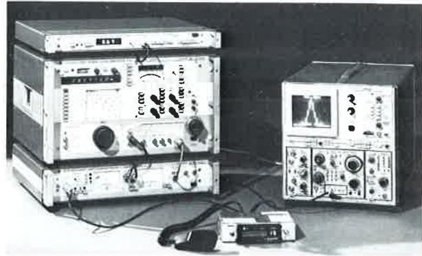
Test setup comprising Adjacent-channel Power Meter NKS, Signal Generator SMDU 06 and AM Unit SMDU-Z1
