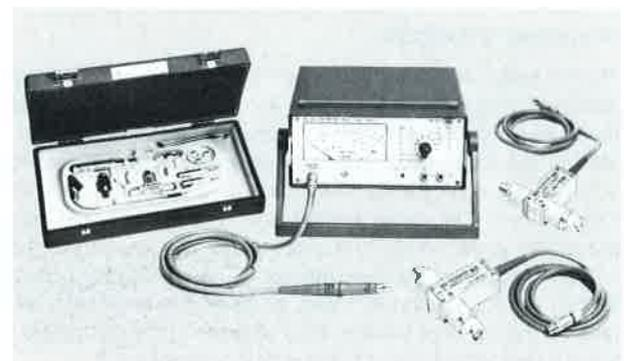
**Input Impedance of RF probe.** The input impedance of the RF probe is given by the input capacitance  $C_{in}$  (see to the right) and the parallel input resistance  $R_p$ , which is dependent on the test voltage (100 k $\Omega$  to 1 M $\Omega$  between 1 mV and 10 V) and, above 3 MHz, also on the frequency.
