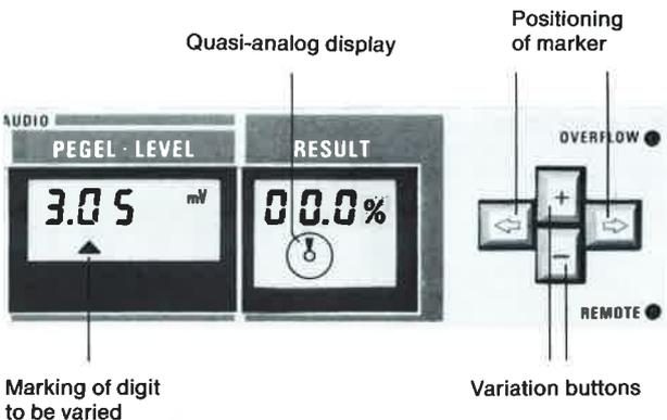
Buttons on mobile tester for varying any desired digit of level and frequency of RF and AF generators as well as modulation section
