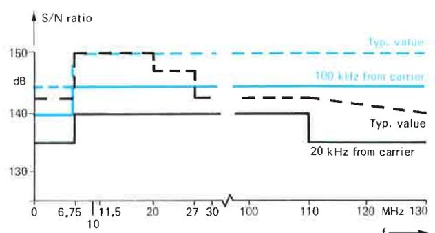
Signal-to-noise ratio referred to 1 Hz as a function of carrier frequency and offset from carrier
