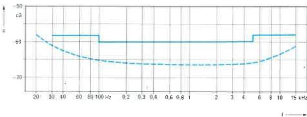
Stereo separation of the Precision Stereocoder MSC 2 between the right and left channels; full line: guaranteed values; dashed line: typical values
