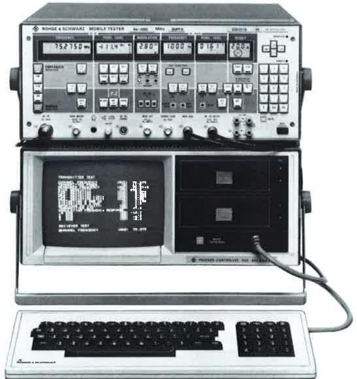
Mobile Tester SMFP2 with Process Controller PUC
