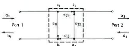
For measuring s-parameters one directional coupler for the input quantities, one for the output quantities and a third (reference coupler) for the voltage required to form the ratio are needed.
