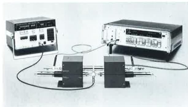
Reflection measurement using Signal Generator SMS, Vector Analyzer ZPV and Directional Couplers ZPV-Z3
