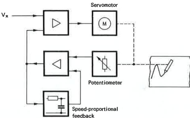
Simplified diagram of potentiometer-type recorder
