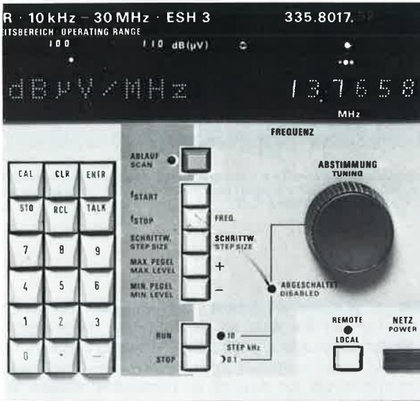
Front panel section with controls for frequency entry and recall
