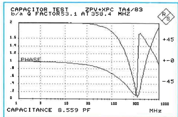
Printout of chip-capacitor measurement
