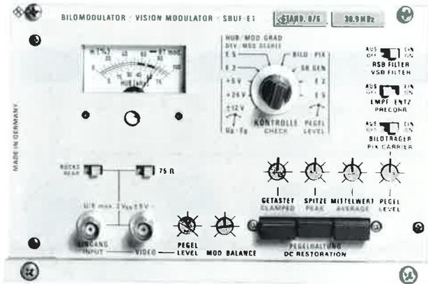
The carrier frequency is supplied by an internal crystal oscillator or an external signal source. A switch is fitted for **double-sideband modulation** (1-dB bandwidth  $\pm 8$  MHz) or – via a group-delay-equalized filter – **vestigial-sideband operation**.
