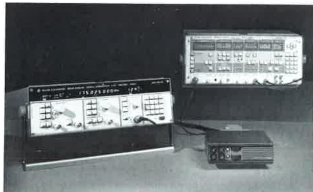
SMPC used as interference source in two-source measurements on RT unit
