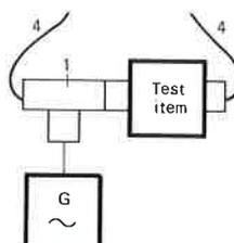
Transmission-factor measurements (calibration: without test item)
