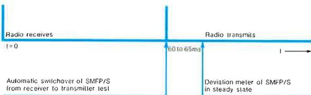
Timing sequence for testing transceivers that send an acknowledgement signal
