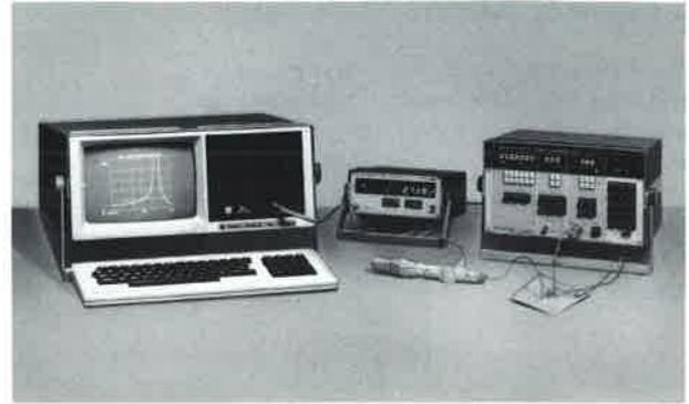
Program-controlled frequency measurement with Signal Generator SMS, Process Controller PUC and Millivoltmeter URV4
