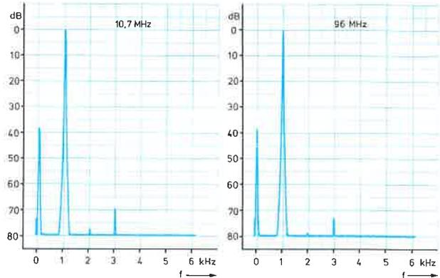
Typical FM distortion at 75 kHz deviation, left:  $f_{\text{carrier}} = 10.7 \text{ MHz}$ , right:  $f_{\text{carrier}} = 96 \text{ MHz}$
