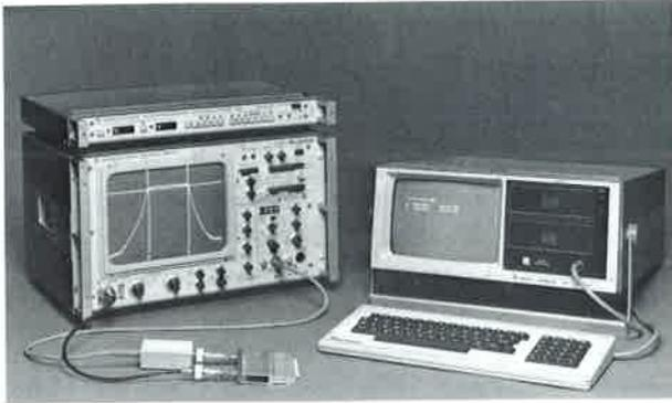
Computer-aided sweep test assembly with Polyskop SWOB 5, Digital Display Store BDS and Process Controller PUC
