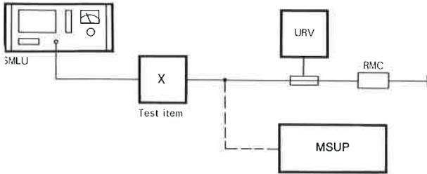
Test setup for intermodulation and crossmodulation measurements
