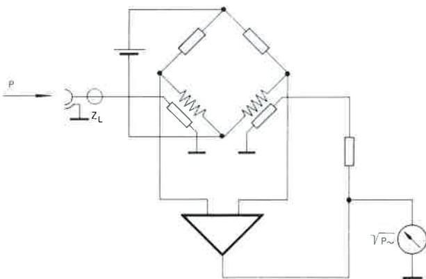
Power measurement using temperature-dependent resistors in a bridge circuit
