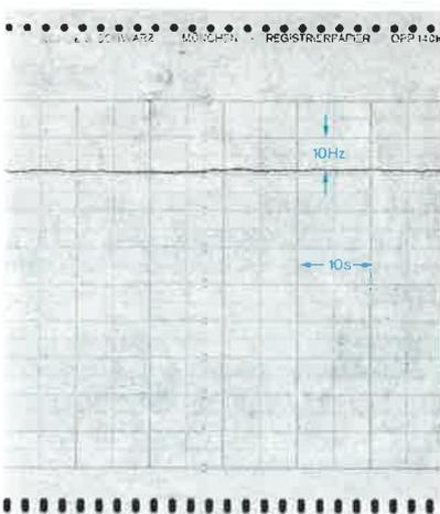
Quality of SMUV signal at 20 MHz: short-term carrier stability (unsynchronized)
