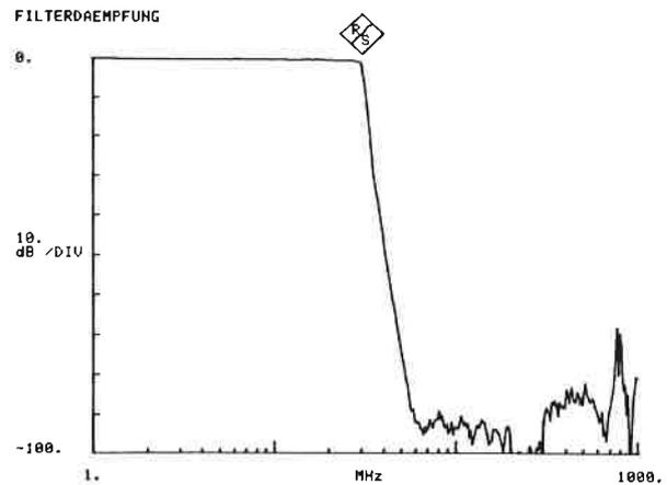
Measured filter response output by computer
