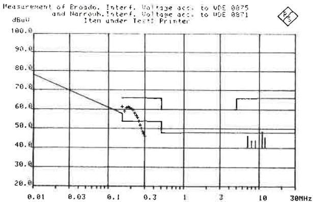
Radio-Interference measurement according to VDE, CISPR and FCC: rapid peak and average measurements permit distinction of wideband and narrowband interference. Only wideband interference near limit value is measured to CISPR to reduce overall measurement time (approx. 8 min for one phase of power lead); limit curves to VDE 0875 (grade N) and VDE 0871 (class B)
