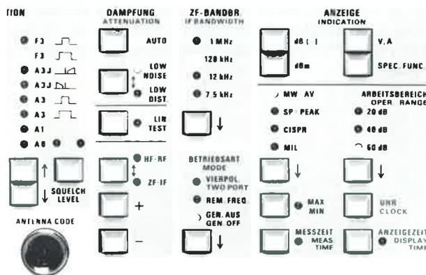
Front-panel section with operating controls for demodulation, attenuation, IF bandwidth and display
