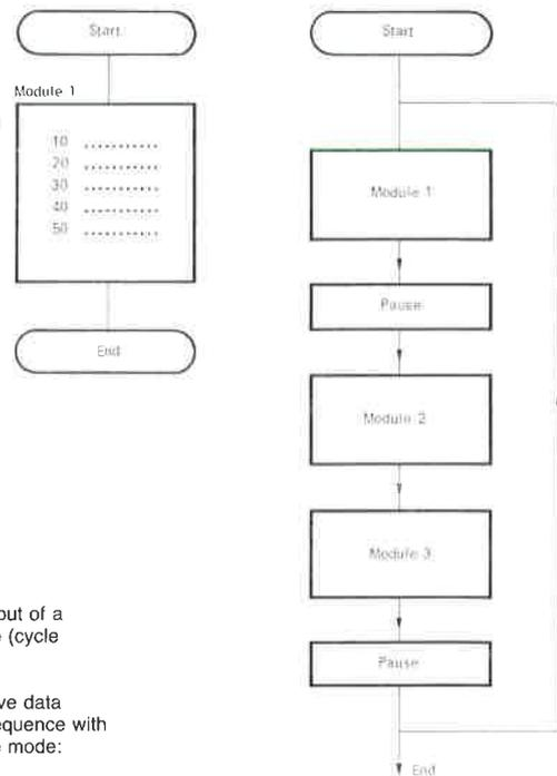
Left: data output of a single module (cycle mode: single)
