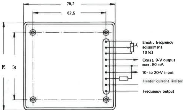
Pin assignments of Crystal Oscillators XSE and XSF
