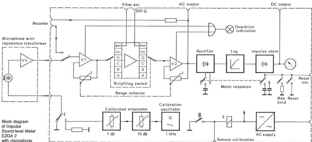
**Microphone.** The capacitor-type Standard Microphone MKPM (page 283) can be electrically heated from the EZGA 2 and is thus optimally protected against environmental influences. For fixed outdoor use, the microphone can also be supplied with a weather shield. The low output impedance of the MKPM permits the use of connecting cables up to 100 m long.
