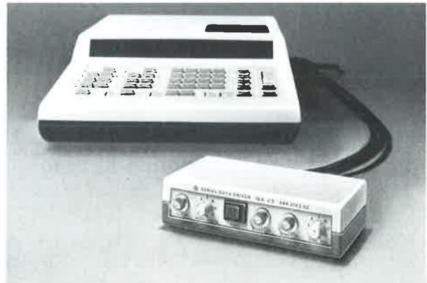
IGA with Serial Data Driver IGA-Z9 for bit-serial data generation (two Serial Data Drivers can be connected simultaneously)
