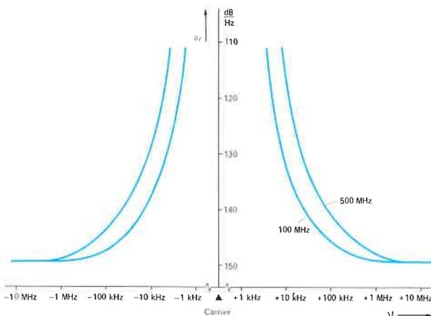
Signal-to-noise ratio of SMDU carriers 100 MHz and 500 MHz at 1-Hz test bandwidth
