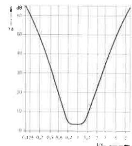
Typical filter characteristic of a PBO
