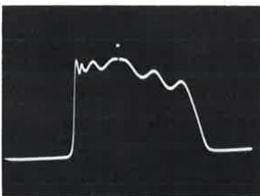
Swept-frequency measurement on a filter with frequency-response display and centre-frequency marker on screen of Analog Display
