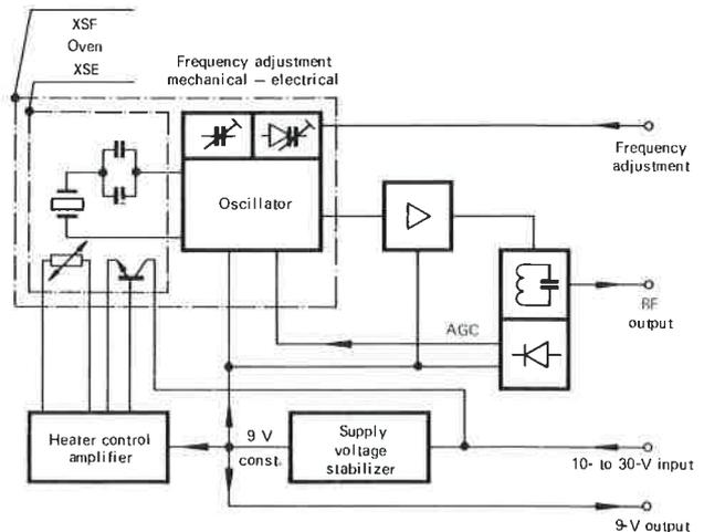
Block diagram of Crystal Oscillators XSE and XSF
