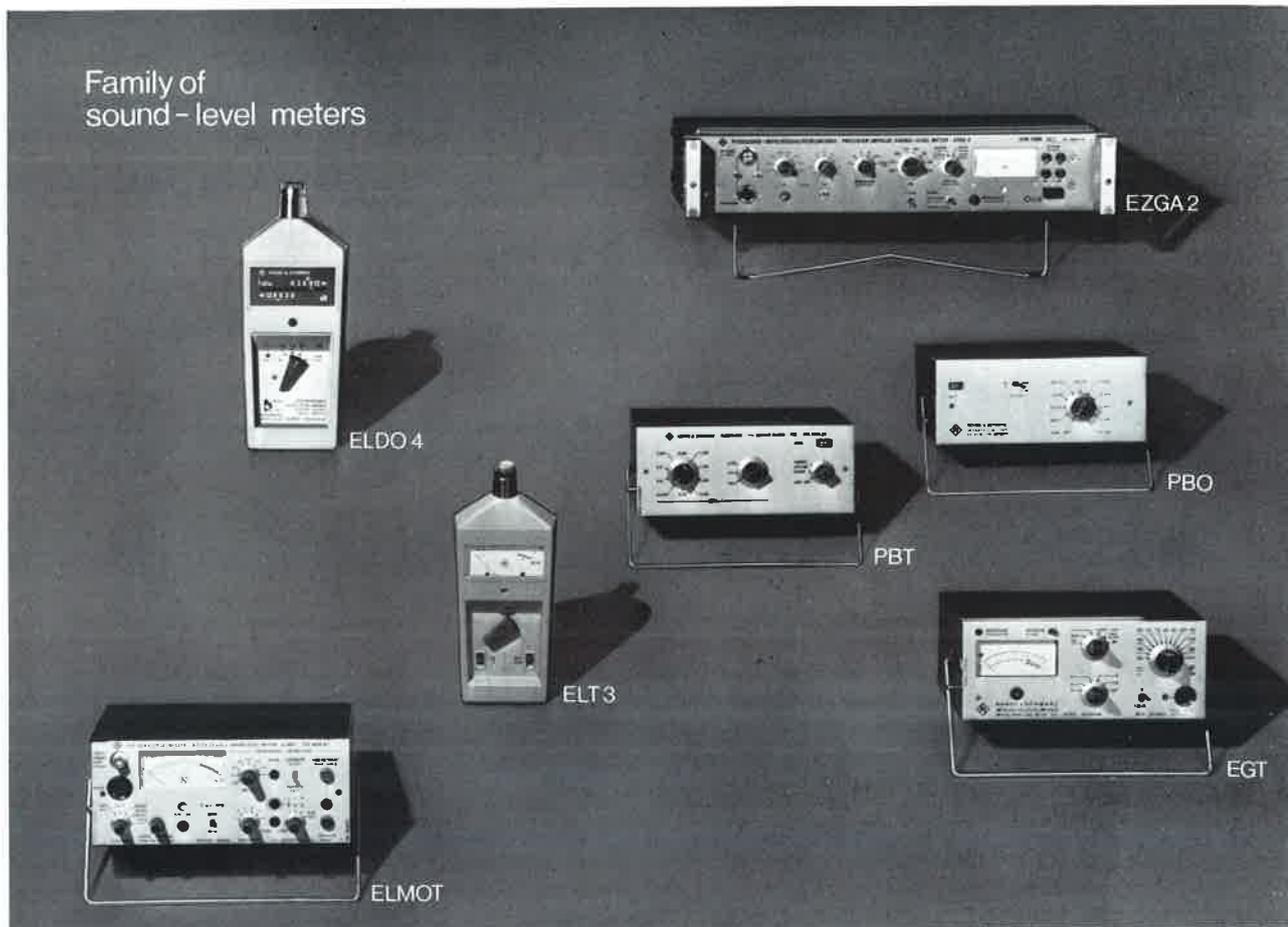
All instantaneous-value reading R&S sound-level meters are type-approved, i.e. they are admitted for calibration by PTB (Federal-German Office of Standards).
