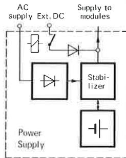
The Power Supply XSRM-Z contains a maintenance-free NiCd cell battery which feeds the instruments connected (e.g. XSRM or XSD2) for one to six hours in the case of AC supply failure. The XSRM-Z delivers a peak current of 1.6 A.
