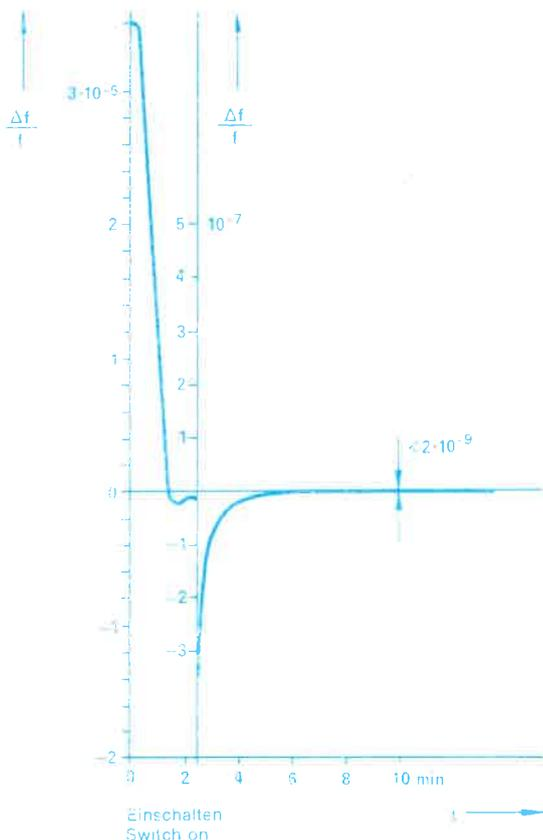
Warmup response of XSE using 5-MHz crystal (3rd harmonic) referred to values obtained after 60 minutes of operation
