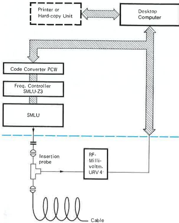
Block diagram of test assembly for RF cables
