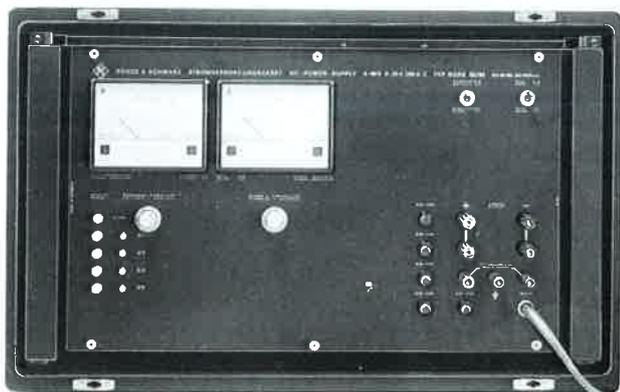
Voltage and current are set by means of high-resolution ten-turn potentiometers and indicated on separate panel meters. The power supplies are fitted with remote-sensing sockets for output-lead voltage-drop compensation. A quiet cooling fan with two-stage thermostat-controlled operation is incorporated.
