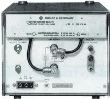
Rear of UPGR with Telephone Weighting Filter UPGR-Z1 attached
