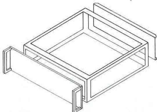
19" basic rackmount in design 80; frame, front and rear panels
