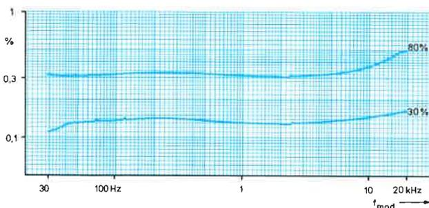
Typical AM distortion of the SMUV at modulation depths of 30% and 80%
