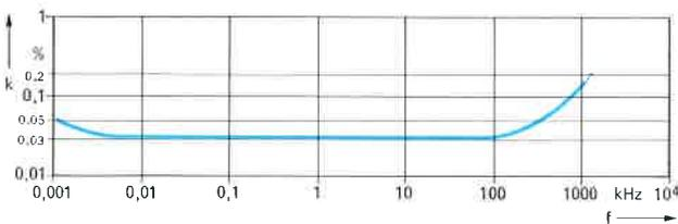
Guaranteed distortion limits for maximum output EMF of 10 V<sub>rms</sub> (k=distortion)
