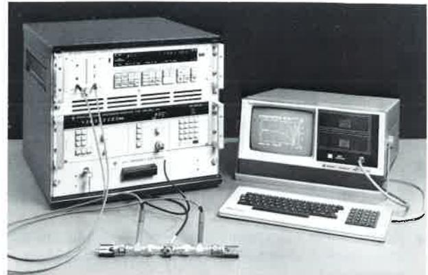
RF-component tester with test adapters for Q and capacitance measurements on chip capacitors
