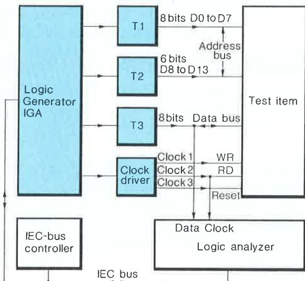
Example for combination of logic generator and logic analyzer (for text see under application examples)
