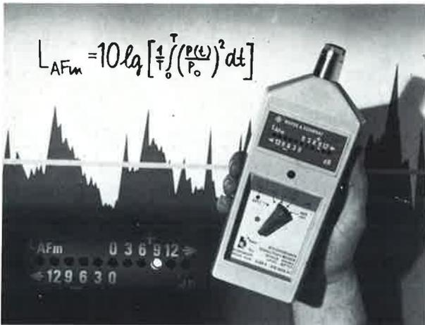
**Integrating sound-level meters** have gained special importance in the last few years. They evaluate the varying sound level occurring over a predetermined time, e.g. a work shift, and form the mean sound level whose annoyance effect is assumed to be equal to the actual sound effect. The mean level is used for comparison of the different noise levels.
