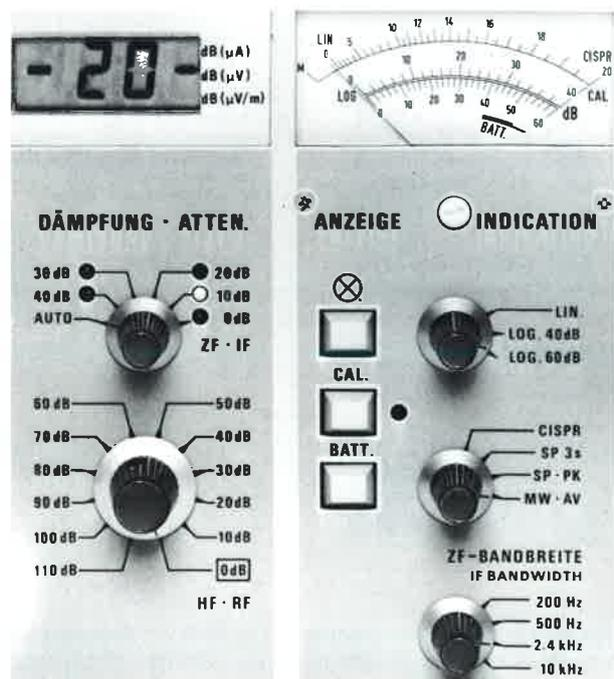
Front panel section with controls for level, bandwidth, weighting and display
