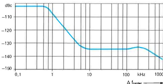
Typical values of SSB phase noise,  $f = 120\text{ MHz}$
