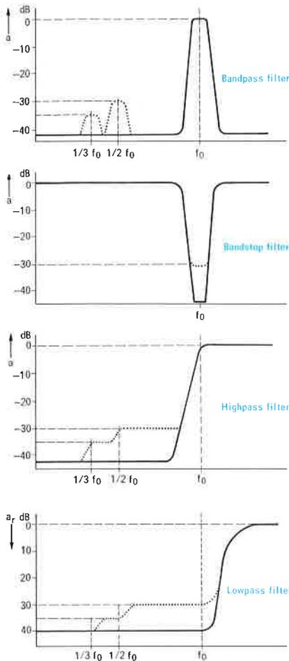
**Bandpass filter.** When reaching an integral submultiple of the passband frequency, the corresponding harmonics are allowed to pass through the filter and are evaluated. Below the passband, apparent attenuation dips are produced. The difference between the peak attenuation of these dips and the true passband attenuation of the filter corresponds to the suppression of the related harmonic.
