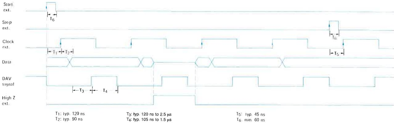
Timing diagram of data output (single module)
