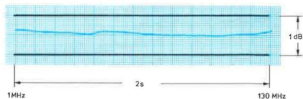
Typical frequency response of Sweep Oscillator SMUV-B5
