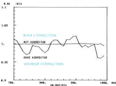
Reflection measurement with and without three-point error correction
