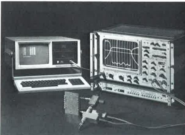
Wideband sweep assembly: Polyskop SWOB 5 (equipped with Logarithmic Amplifier SWOB5 E3), Digital Display Store BDS and Process Controller PUC (for data storage)
