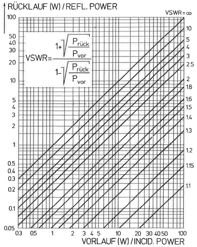
Graph to derive VSWR from incident and reflected power (provided on the rear panel of each instrument)
