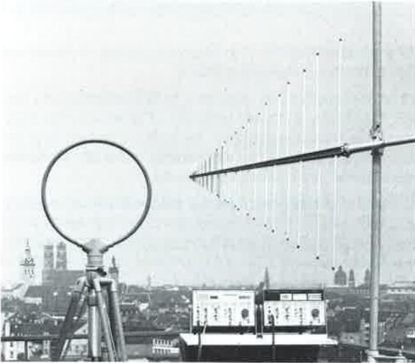
VHF-UHF Field-strength Meter HUF for propagation measurements, measurement of radiation patterns and interference field strength
