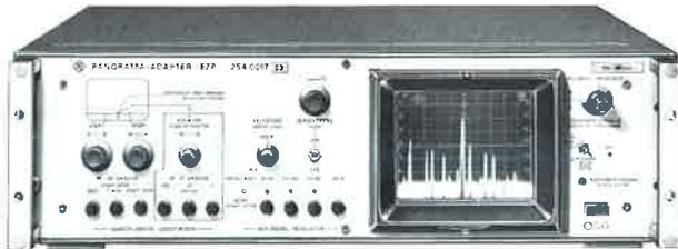
The **Panoramic Adapter EZP** in conjunction with a suitable receiver, such as the ESU 2 or ESM 2, permits spectral display within a particular frequency range. The screen display supplies information on band occupancy, and on the level, modulation and frequency spacing of the individual signals.
