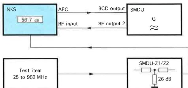
NKS in conjunction with Radiotelephone Test Assembly SMDU
