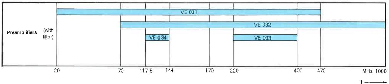
The weather-protected **Preamplifiers of the VE 03. series** are used to compensate for the line losses between the antenna and the receiver, e.g. in **radiomonitoring** and **air traffic control** systems.
