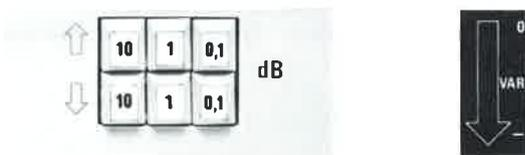
The 0.1-dB keys are used for noninterrupting electronic fine level adjustment. The state of the electronic level variation can be seen at a glance from the LED array
