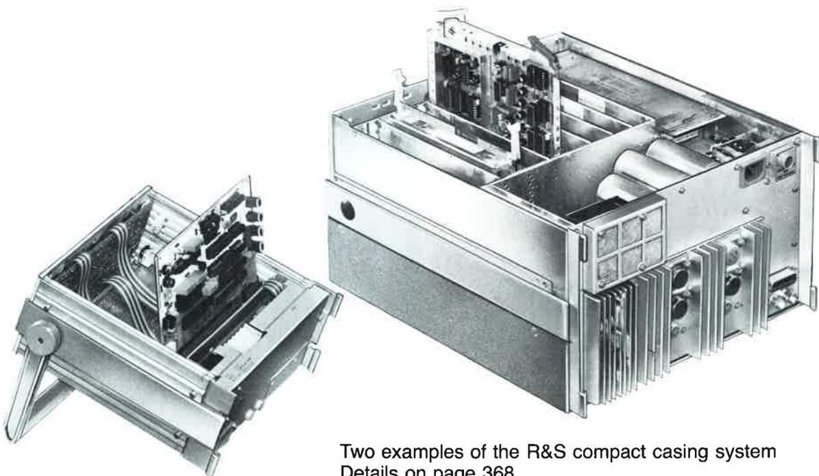
Two examples of the R&S compact casing system
