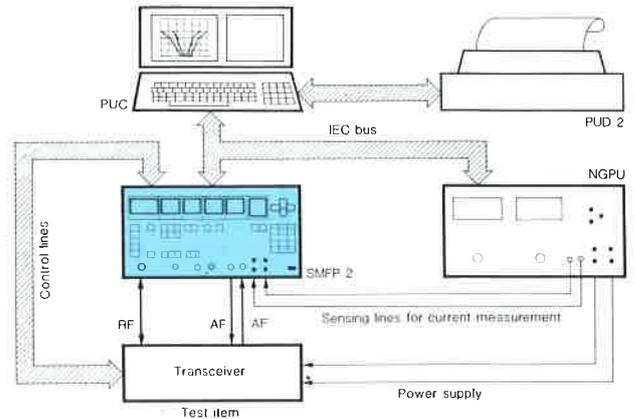
Fully automatic transceiver test assembly with Mobile Tester SMFP2, Process Controller PUC, Universal Printer PUD2 and Programmable Power Supply NGPU
