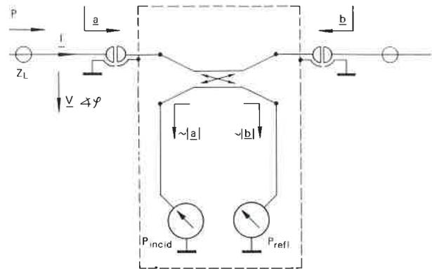
Power measurement using directional coupler
