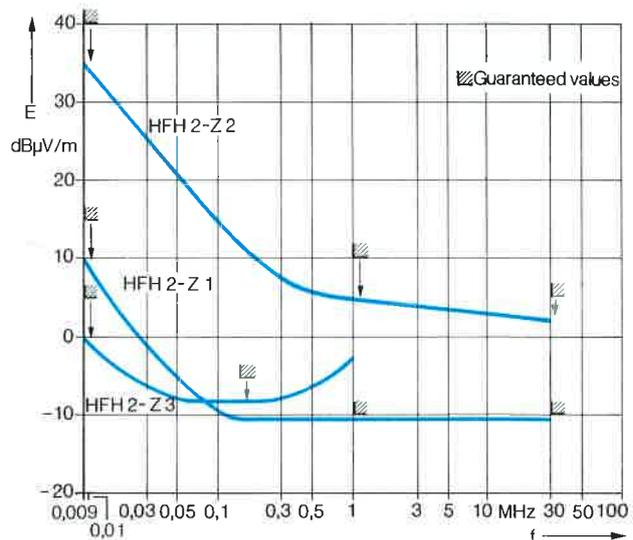
● Active **Loop Antenna HFH 2-Z2** for measuring the magnetic field-strength component
