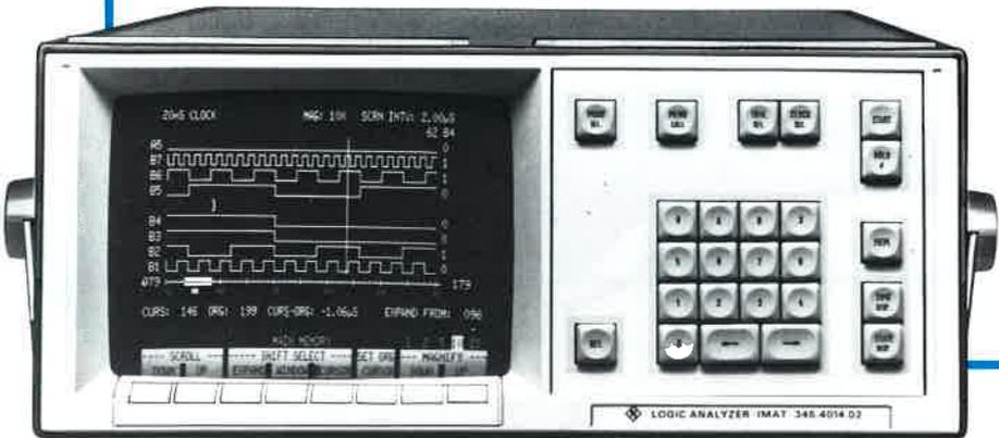
Logic Analyzer IMAT ♦ Sampling rate 100 MHz
