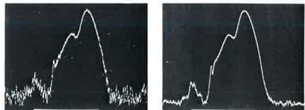
Frequency response display: (left) signal with heavy noise component and (right) after taking the average over successive sweep with the corresponding BDS option
