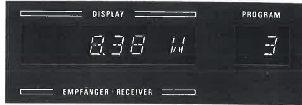
Display of measured value: example power measurement
