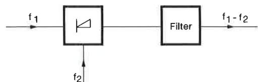
The advantages of this method are the extremely short frequency switching time and the lack of problems when the signal is modulated (FM, AM and SSB).
