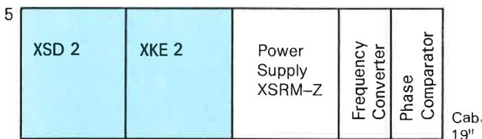
Test assembly for crystal oscillator recalibration; with controlled crystal standard for stationary use only; long-term drift:  $\approx 5 \times 10^{-10}$ /without limit, depending on local receiving conditions
