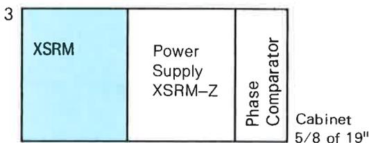
Test assembly for crystal oscillator recalibration, also for mobile use; long-term drift:  $<1 \times 10^{-11}$ /month
