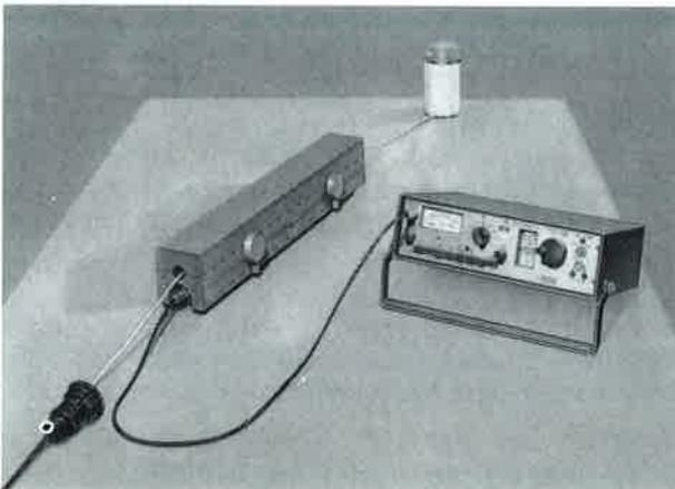
Test setup consisting of VHF Field-strength Meter HFV and Absorbing Clamp for the measurement of interference power
