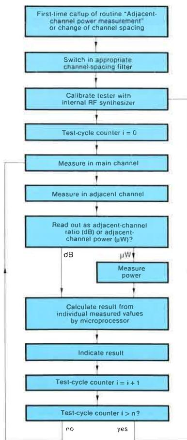
Comprehensive automatic internal test routines offer extreme operating ease combined with high accuracy: simplified flow chart for automatic test routine for adjacent-channel power measurement
