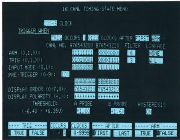
Setting the trigger linkage
