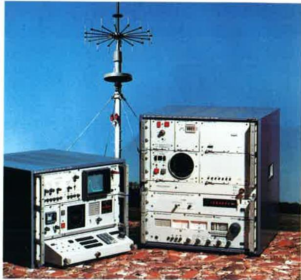
VHF-UHF Broadband Doppler Direction Finder PA 005 for radiomonitoring systems covering 20 through 1000 MHz
