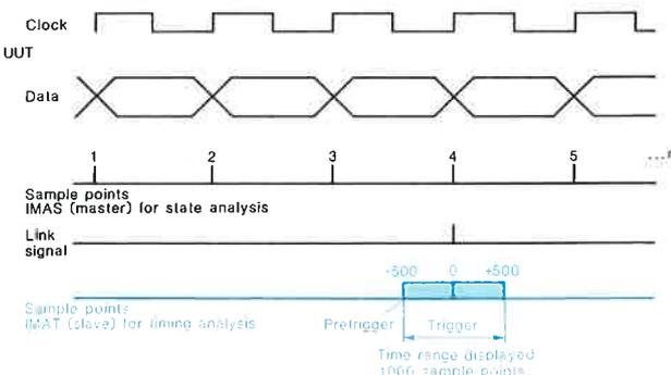
Simultaneous logic state and timing analysis
