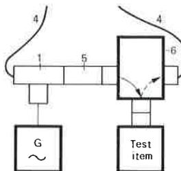
Impedance measurements with **VSWR bridge** (calibration: shortcircuit in place of test item)
