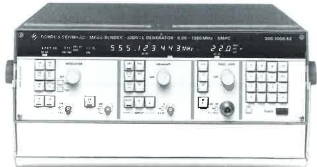
For the first time a synthesized generator with this high degree of spectral purity features also AM, FM and  $\phi$ M characteristics of maximum quality. The FM distortion of less than 0.1% and an adjacent-channel crosstalk which is down more than 56 dB permit measurements even on high-grade stereo receivers to be performed.
