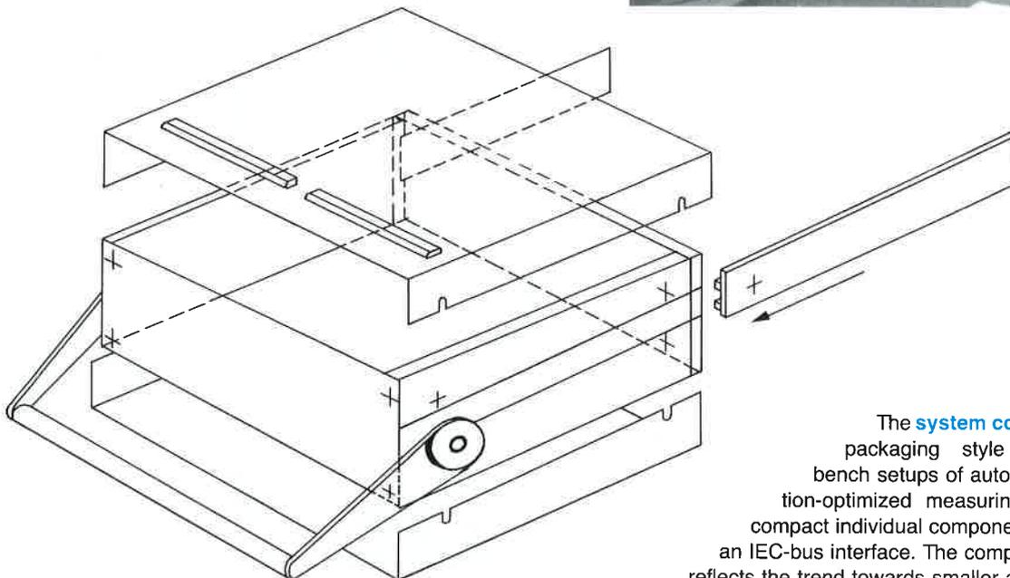
The **system compatibility** of this packaging style enables simple bench setups of automatic and application-optimized measuring systems, using compact individual components, e.g. units with an IEC-bus interface. The compact casing system reflects the trend towards smaller assembly units.
