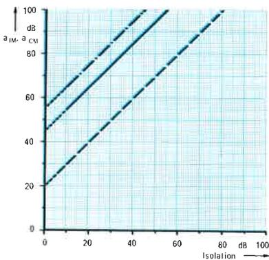
Intermodulation and crossmodulation suppression  $a_{IM}$  and  $a_{CM}$  of SMLU as a function of isolation; **solid line:** three-signal IM suppression referred to sync peak; **dashed line:** two-signal IM suppression referred to carrier; **chain-dotted line:** CM suppression
