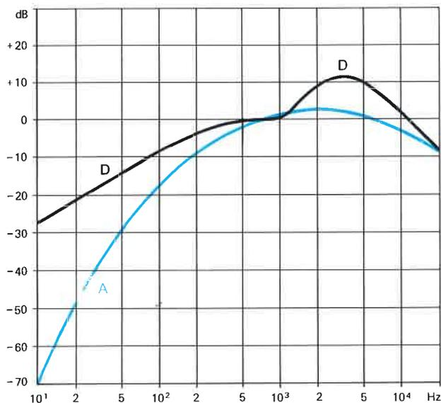
Relative attenuation of weighting networks referred to 1 kHz
