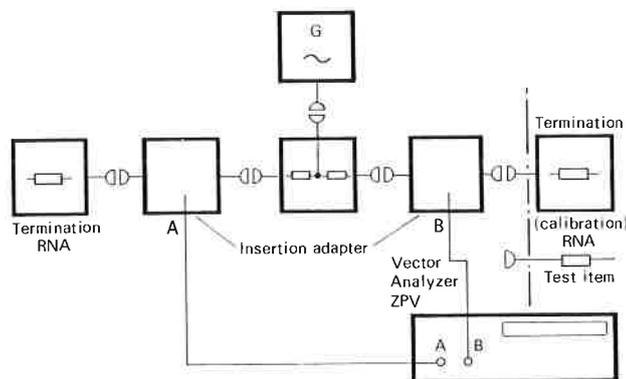
Two-port measurement based on the voltage method
