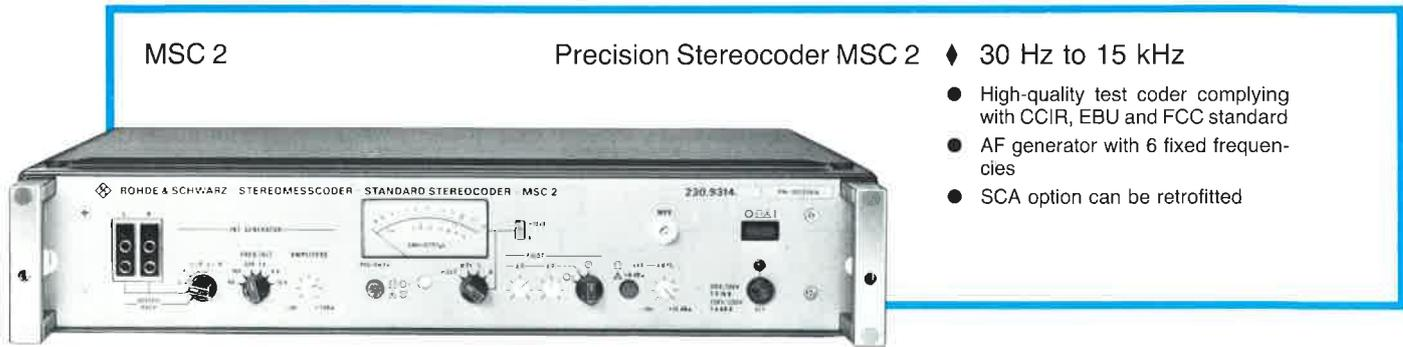
The **Precision Stereocoder MSC 2** produces the standard multiplex signal with **high precision**.
