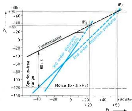
2nd and 3rd order intercept points (IP<sub>2</sub> and IP<sub>3</sub>) of Preamplifier VE 031; P<sub>1</sub> = input level, P<sub>0</sub> = output level
