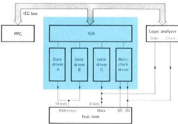
Digital functional test in multi-clock mode (using IGA, logic analyzer and process controller)
