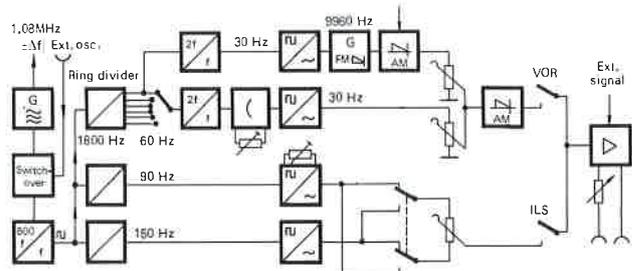
Generator section of the VOR/ILS Unit; processing of modulation signals
