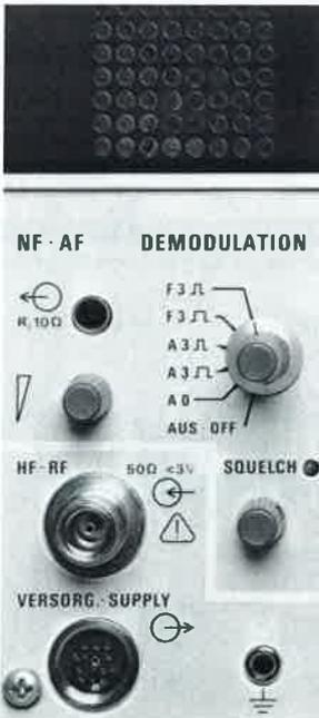
Front-panel section: demodulation and AF setting; RF input, squelch and power supply for Current Probe
