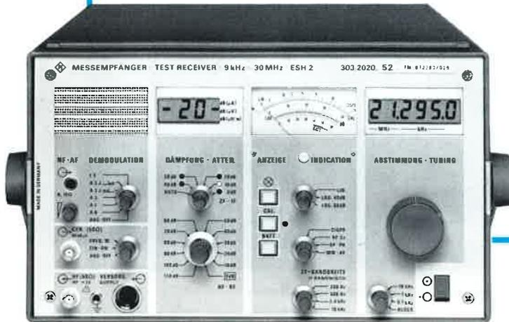
The **ESH 2** is a manually operated, sensitive and overload-protected test receiver offering a very wide dynamic range and maximum ease of operation. Compact construction, the wide range of power supplies that can be used, and low power consumption make the receiver suitable for use in fixed stations as well as for mobile and portable applications.
