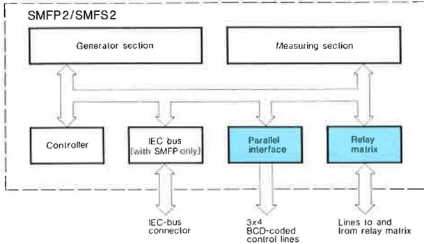
Basic diagram of SMFP2 and SMFS2 subdivided into generator, measuring and control sections; blue: standard with SMFP2, optional with SMFS2
