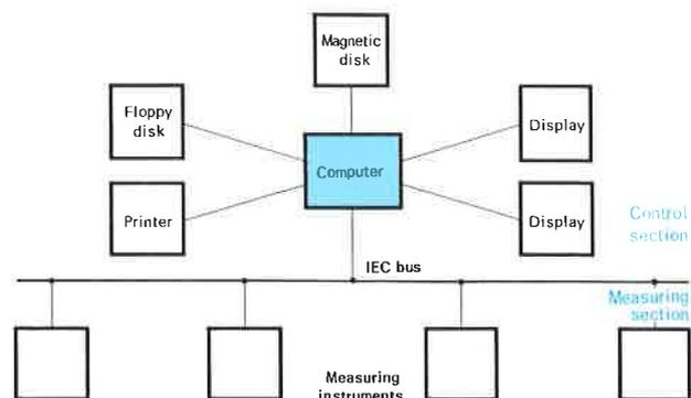
Block diagram of test assembly with computer control
