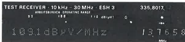
Front-panel section with frequency display and alphanumeric display, e.g. for results of measurements
