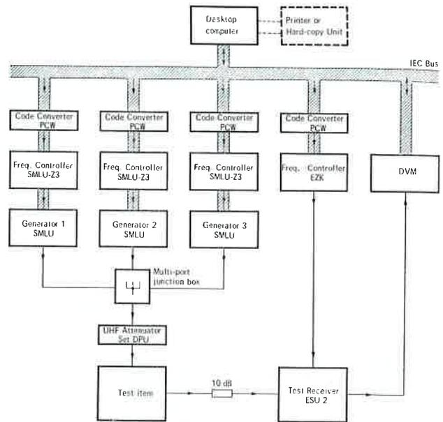
Block diagram of the Automatic RF Test Assembly for intermodulation and crossmodulation measurement
