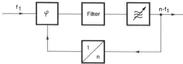
Phase-locked loops have the advantage that they are largely free from spurious responses since these are filtered out by an AF filter in the control voltage path. When using suitable dividers any integral frequencies can be selected, so the PLL technique is ideal for generating the main frequency range of synthesizers. With a control response that is fast enough and a suitable reference frequency particularly low-noise output signals can be produced. Frequency modulation can be transferred.
