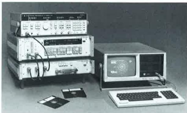
Computer-controlled network analyzer assembly comprising Vector Analyzer ZPV, Sweep Generator SWP (synthesizer), S-parameter Test Adapter ZPV-Z5 and Process Controller PUC
