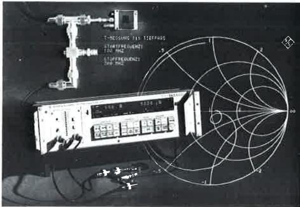
Vector Analyzer ZPV fitted with Tuner ZPV-E3 used for filter measurement according to T-junction method
