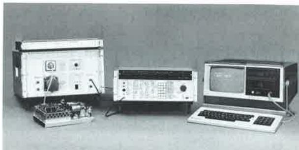
Automatic interference-voltage measurement with programmed phase-switching: Test Receiver ESH 3, Artificial Mains Network ESH 2-Z5, Process Control PUC and Code Converter PCW
