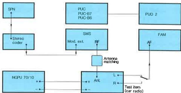
Block diagram of automatic test system for stereo car radios consisting of Generator SPN 1 Hz to 1.3 MHz, Signal Generator SMS 0.1 to 520 MHz, Modulation Analyzer FAM, Power Supply NGPU 70/10, Process Controller PUC and Universal Printer PUD 2
