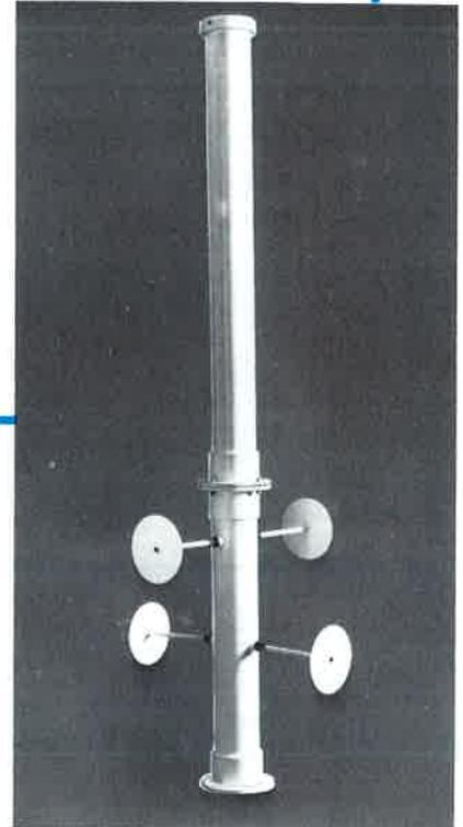
The **Active Antenna System HE 115** is made up of the Active Receiving Dipole HE 101 (2 off) and the Active Vertical Dipole HE 109 (see illustration on the right).
