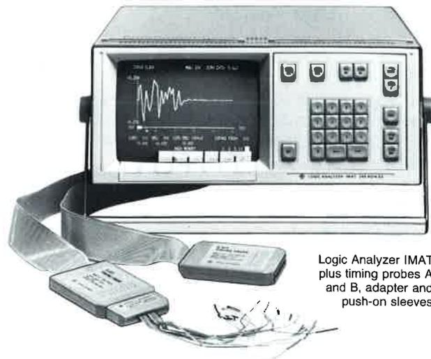
Logic Analyzer IMAT plus timing probes A and B, adapter and push-on sleeves
