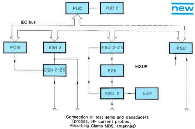
Block diagram of automatic HF-VHF-UHF system consisting of Test Receiver ESH 3, VHF-UHF TEST Equipment MSUP, Code Converter PCW, Artificial Mains Network (LISN) ESH 2-Z5, Process Controller PUC and Universal Printer PUD 2
