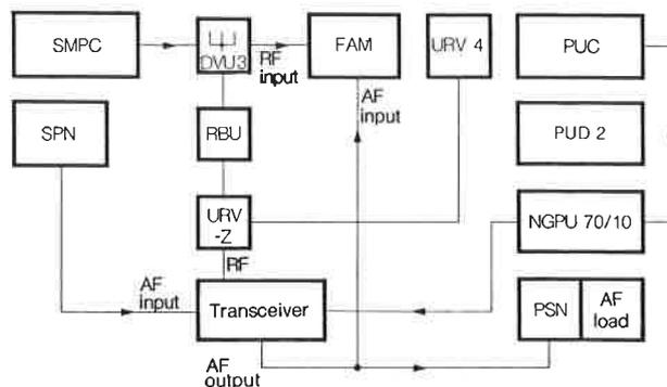
Block diagram of reference system for transceiver test
