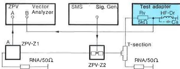
Block diagram of RF-choke test system
