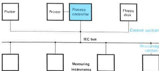
Block diagram of automatic test assembly
