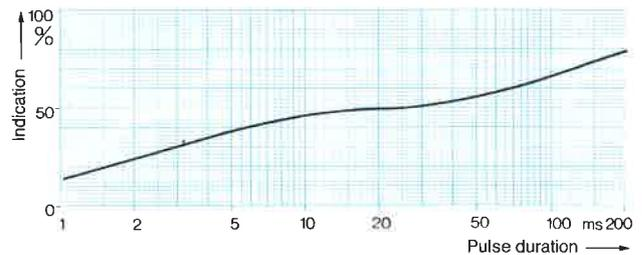
Peak indication as a function of pulse duration in measurements with single bursts of a 5000-Hz sinewave signal (amplitude corresponds to 100% indication with continuous signal)
