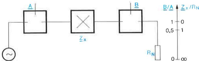
Result from  $B/A$  ratio measurement as a function of impedance  $Z_x$  (when using voltage division principle)
