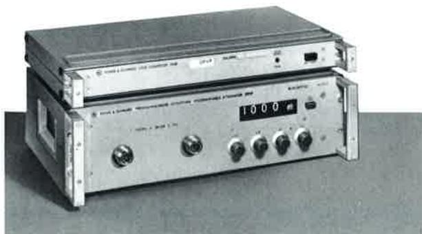
Programmable Attenuator DPVP plus Code Converter PCW (for programming via IEC bus)
