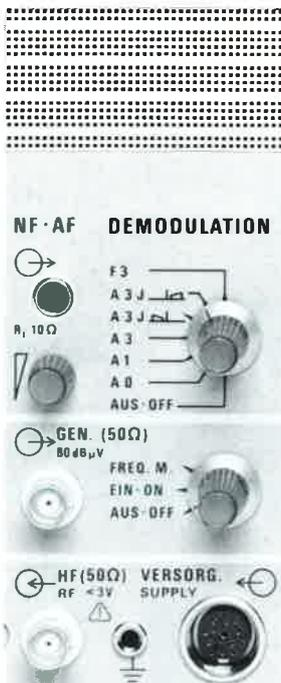
Front-panel section: demodulation and AF settings; output for calibration signal and frequency measurement; RF input and power supply connection
