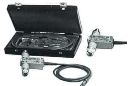
**Input impedance of RF probe.** The input impedance of RF probe is given by the input capacitance  $C_{in}$  (see to the right) and the parallel input resistance  $R_p$ , which is dependent on the test voltage (100 k $\Omega$  to 1 M $\Omega$  between 1 mV and 10 V) and, above 3 MHz, also on the frequency.
