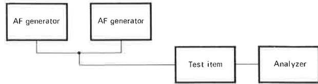
AF distortion measurement by the difference-frequency method
