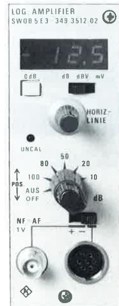
Front panel of Logarithmic Amplifier plug-in SWOB 5 E3
