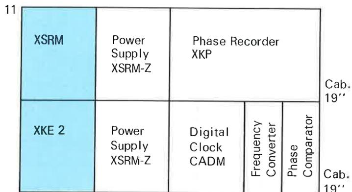
Controlled atomic frequency and time standard, basic equipment for institutes and laboratories requiring precise frequency and time signals
