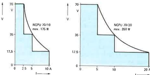
Loading characteristics of programmable power supplies NGPU as function of output voltage
