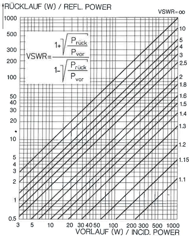
Graph to derive VSWR from incident and reflected power (provided on the rear panel of each instrument)
