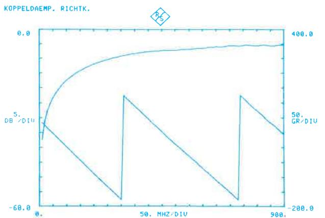
Coupling attenuation of a directional coupler represented in polar coordinates (top) and in cartesian coordinates (bottom); output on hardcopy unit greatly reduced scale)
