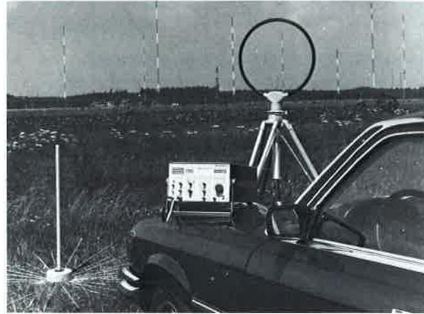
Field-strength Meter HFH 2 for 9 kHz to 30 MHz
