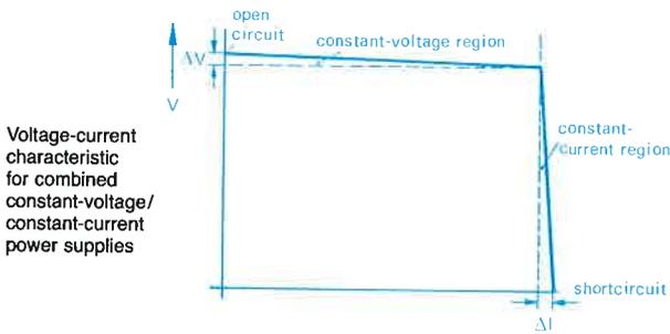
The series NGA and NGAS and the triple supplies NGT and NGL incorporate current limiting which can be continuously adjusted to any value between zero and the rated current. In the NGAS series current limiting can be adjusted to 1,5 times rating (see page 325).
