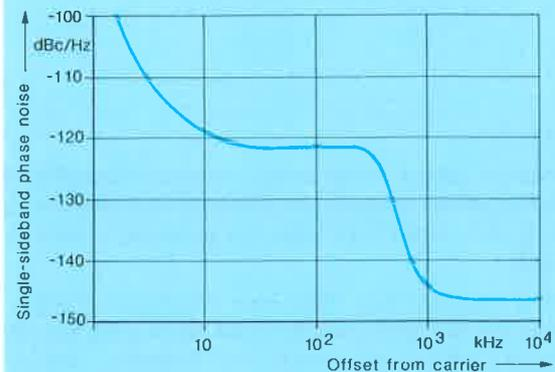
Typical single-sideband phase noise of Signal Generator SMS ( $f_{\text{carrier}} = 360$  MHz)
