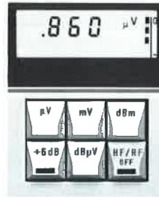
SMFP2/SMFS2 output-level display combined with readout of electronic-attenuator setting plus keys for entry and conversion of physical units
