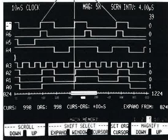
Example of timing analysis with state-domain triggering and disassembler display
