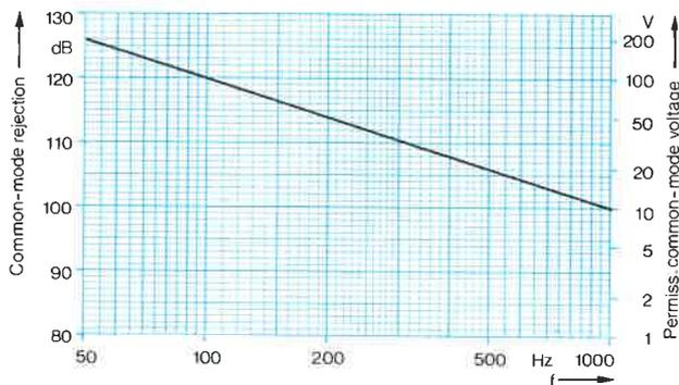
Common-mode rejection and common-mode voltage of UPGR versus frequency
