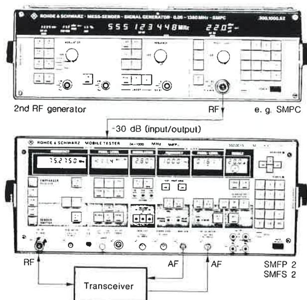
Test setup for two-signal measurements and measurements on repeaters
