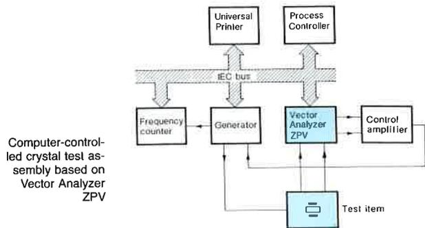
Computer-controlled crystal test assembly based on Vector Analyzer ZPV
