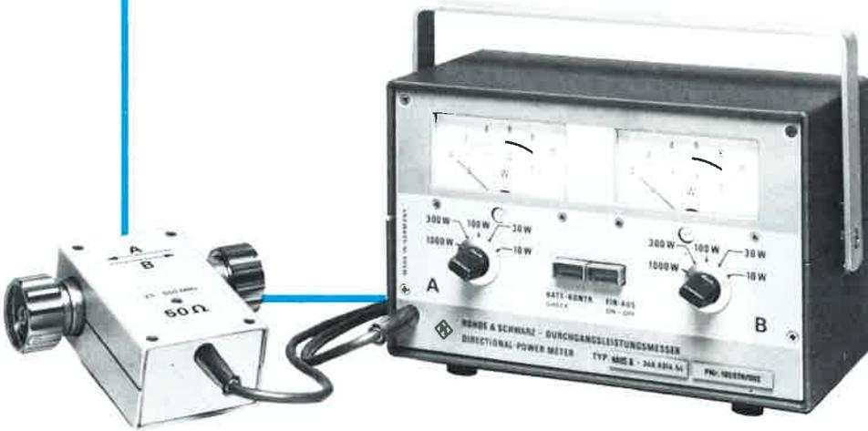
Apart from their higher power rating the **Directional Power Meters NAUS 5 and NAUS 6** are the same in design and performance as the NAUS 3 and NAUS 4 models described on pages 214, 215. Like these they consist of an **indicator** (case with carrying handle) and a separate **measuring head** which can be connected in either direction. The incident and the reflected power are indicated on separate meters in five subranges.
